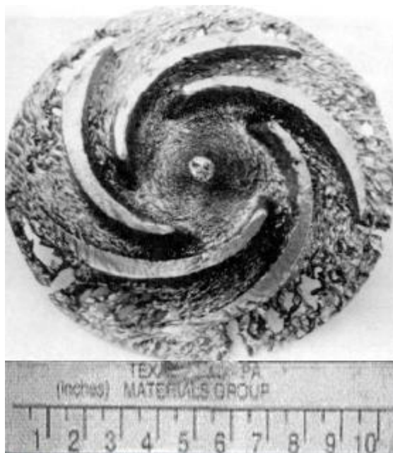
Fig. 8: Erosion-corrosion of a cast stainless steel pump impeller after exposure to hot concentrated sulfuric acid with some solids present. Note the grooves, gullies, waves, and valleys common to erosion-corrosion damage [11].
