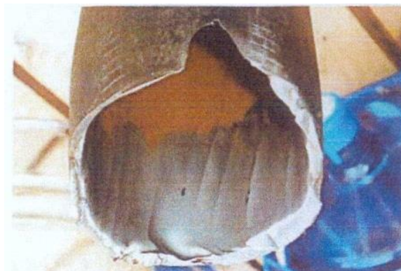
Fig. 66: Oil and gas pipeline after being attacked by stress corrosion cracking [28].
