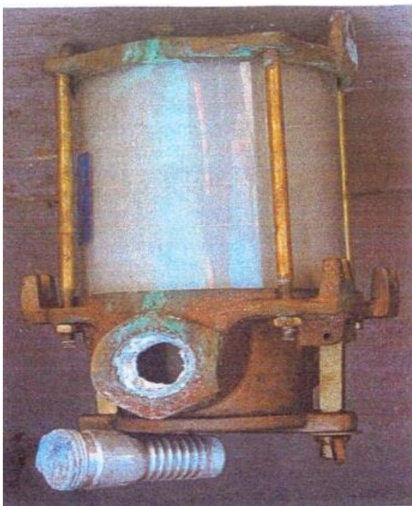
Fig. 63: Galvanic corrosion resulting from placing a bronze sea strainer on an aluminum hose barb [28].
